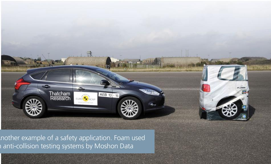
Another example of a safety application. Foam used in anti-collision testing systems by Moshon Data
